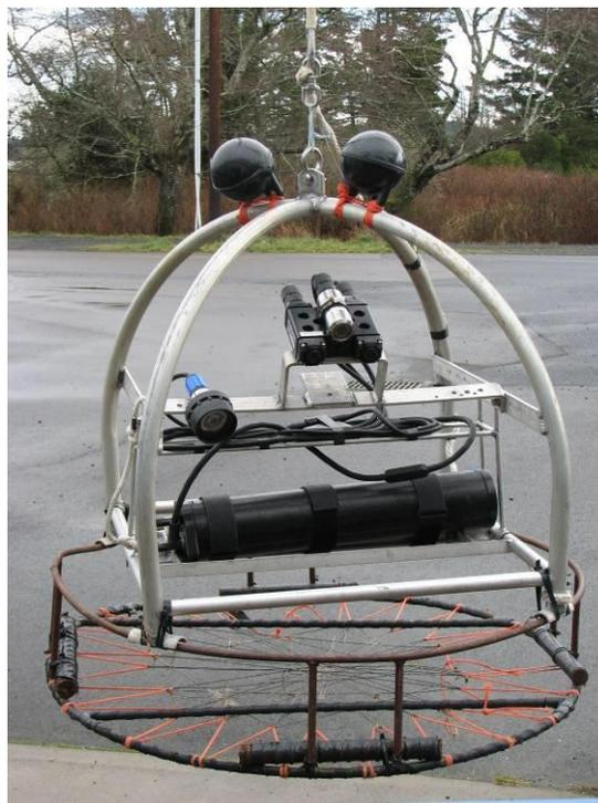
Figure 5. Video lander suspended by buoy line. At top is the breakaway link; at bottom is the breakaway base. Camera, lasers, light and pressure tube are mounted within the aluminum frame.
