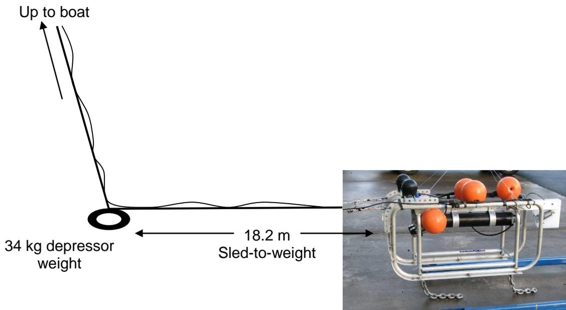
Figure 8. Image of the 2011 revised sled design including a diagram of the towline setup.
