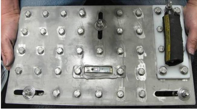
Figure 3. BOP plate with oceanographic instrument mounts (right) and anchor bolts.
