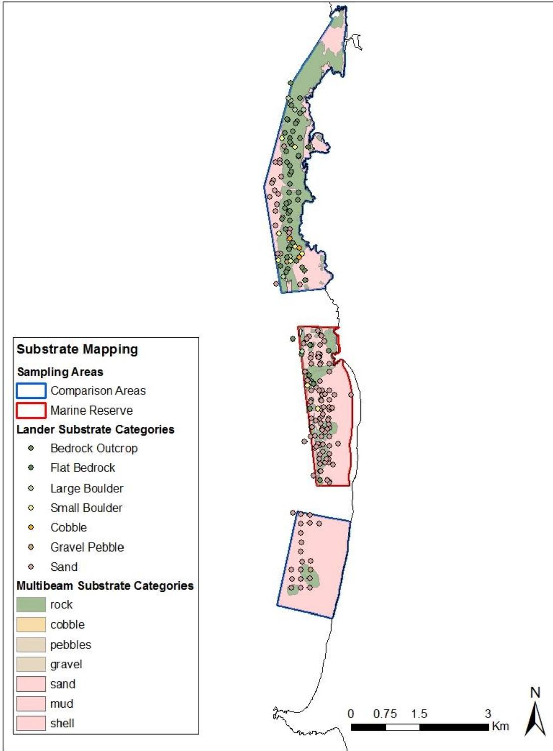
Figure 4. Mapping of substrate types detected by the video lander (circles) and high resolution multibeam survey (polygons). Difference substrate classes were defined for each method; each type of substrate is represented by like colors regardless of sampling method.
